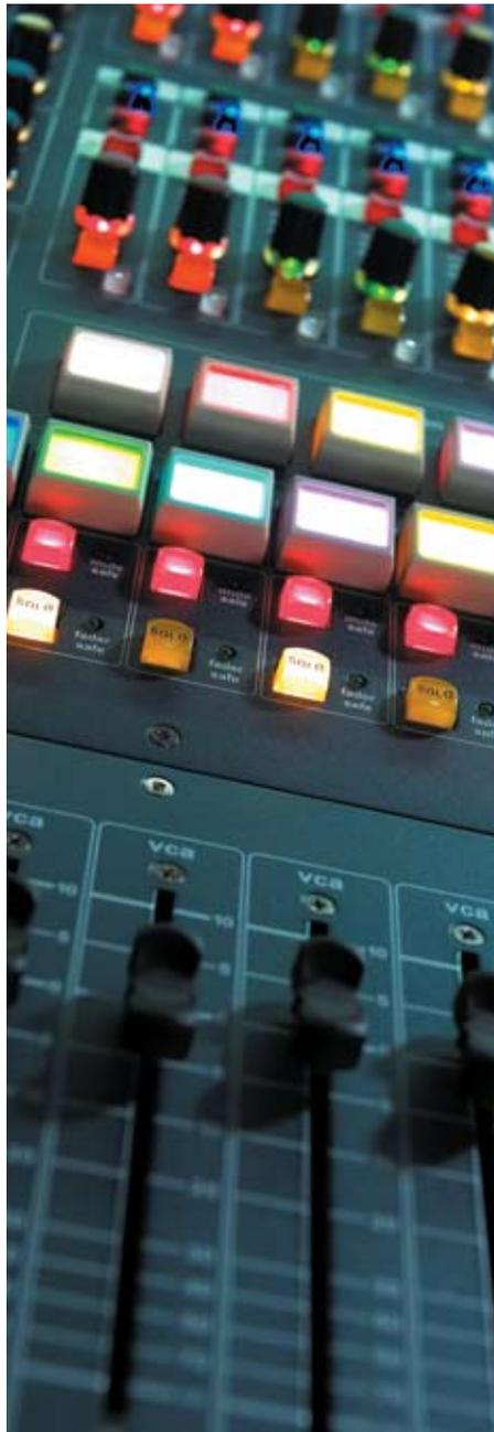
Live sound engineers have typically used colour when navigating mixing consoles, applying different coloured adhesive tape and swapping coloured fader knobs makes console navigation faster, and more intuitive. Midas designers have taken this established principle of channel recognition, and designed the PRO6 Control Centre entirely around this concept, using colour-coded VCA and POPulation groups, as pioneered on the Midas XL8 Live Performance System.
