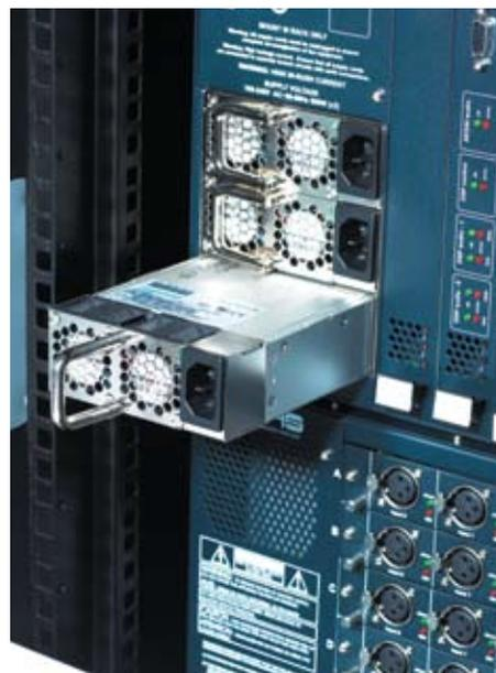
Reliability is a key concern with all Midas products, and all PRO6 hardware elements feature redundant power supplies as standard. The FPGA processing engine is of modular construction, with the option of a spare module which will automatically deploy in the event of an engine module failure (n+1 model).
