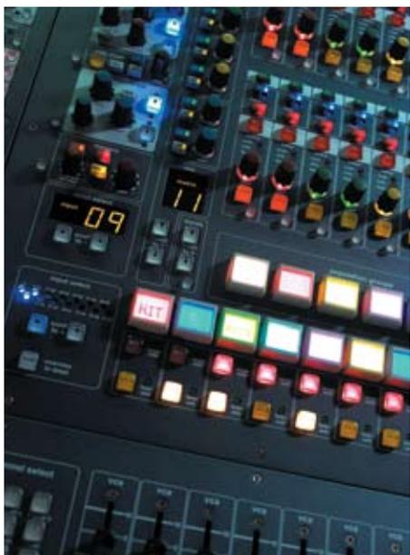
The Midas PRO6 feels, as well as sounds superb. All variable controls on the console are genuine potentiometers, not encoders. These access the FPGA engine through A-D converters, and Midas' custom interpolation algorithms. This means that as well as all audio, all operator input is fully interpolated to ensure a linear, analogue-style, silky smooth "feel" to your mix.
