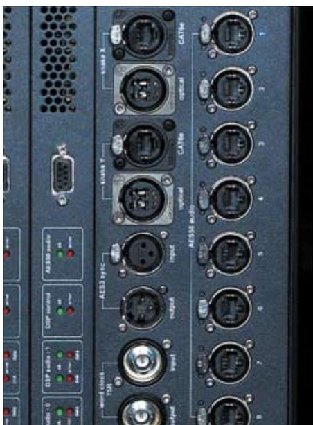
Digital audio transport uses the international AES30 standard, featuring feed-forward error correction which provides superior protection against lost data packets and synchronisation issues when compared to Ethernet-based systems. All links between PRO6 hardware elements support redundant cables for both copper and optical (where available) options.
